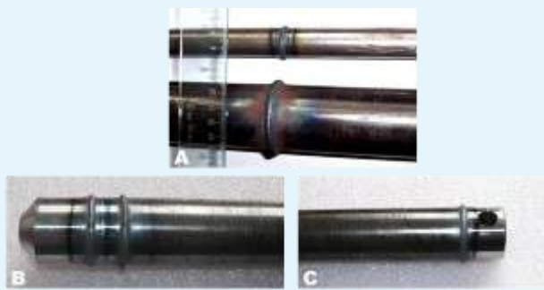
Figure 3: Welded joints of pipes with Ø22mm and Ø51mm (A), Welding to the pipe Ø38x3mm stub and adapter (B) and Welding to the pipe Ø38x3mm with stub with hollow (C)
