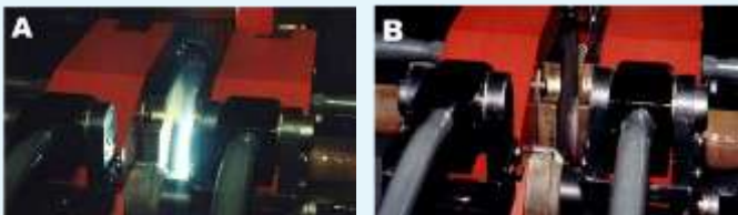
Figure 1: Process of MIAB welding (A) and MIAB welding joint of pipes after upset (B)
