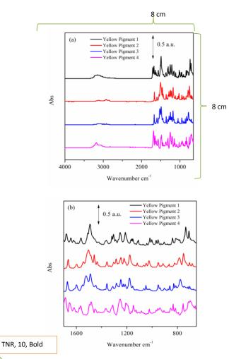
**Figure 2** FTIR spectra of Yellow Pigments 1, 2, 3 and 4 for **a**) whole region and **b**) fingerprint region
