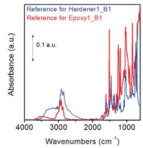
Figure 1 Reference spectra for Epoxy1 and Hardener1
