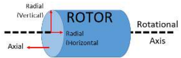
Figure 2 : Figurative representation of vibration measurement directions on a rotating equipment
