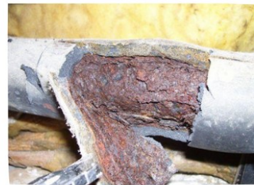
Figure 2: CUI exposed under insulation
