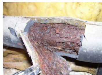
Figure 2: CUI exposed under insulation
