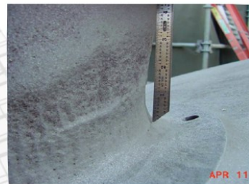
Figure 3: Wall thickness loss due to CUI
