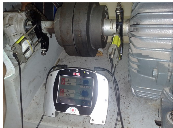
Figure 3: Laser alignment shaft to shaft
