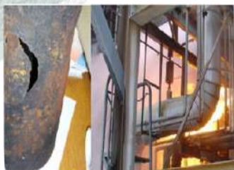
Figure 1: CUI failure on piping leading to a process fire safety incident
