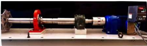
Figure 5: The arrangement for an overhung PMB assembly.
