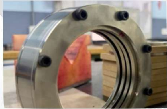
Figure 3: The arrangement of magnetic bearing assembly
